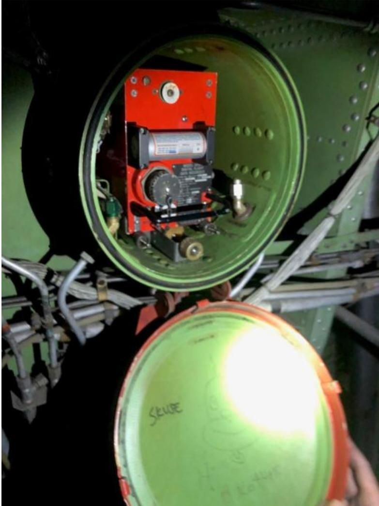
*Flight data recorder. (Photos courtesy of Aircraft Towing Systems World Wide LLC).*
