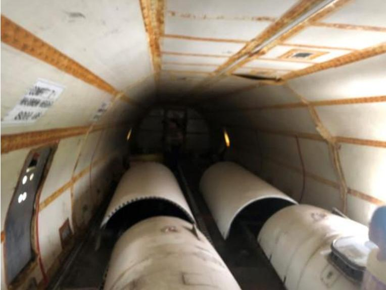
*Two sets of jet engine cowls. (Photos courtesy of Aircraft Towing Systems World Wide LLC).*
