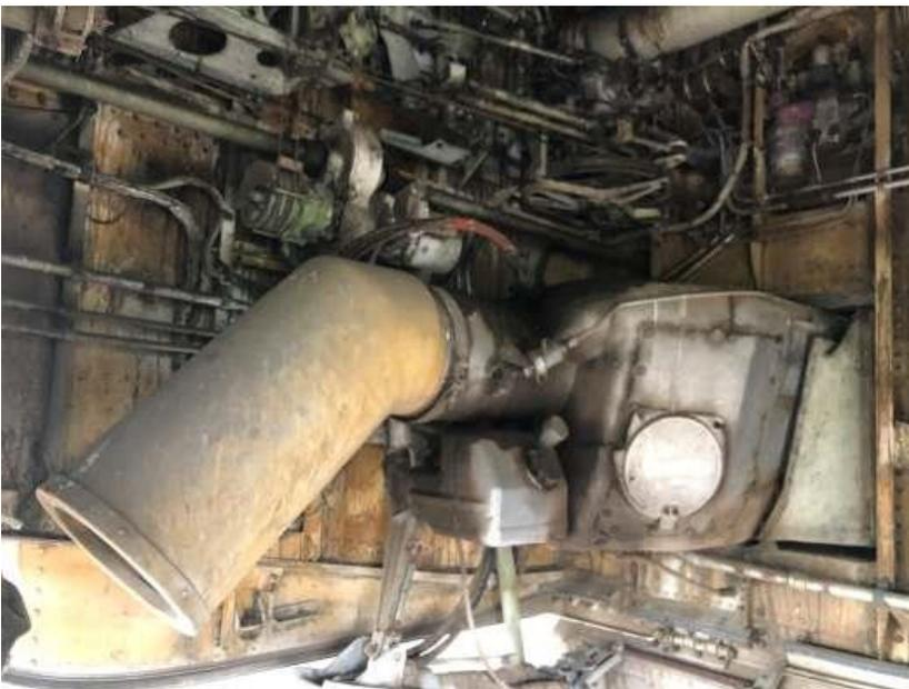
***The intake and fuel control for the auxiliary power unit. (Photos courtesy of Aircraft Towing Systems World Wide LLC).***
